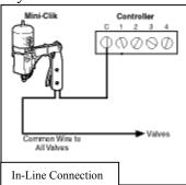
from the sensor to the common wire terminal, and the other to the common wire from the valves. You can also connect the sensor wire in-line anywhere on the common wire, one sensor wire to the common wire to the valves, and the other to the
