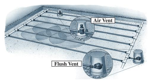
flush valve, which should be located in a valve box at the low end of the system. (See diagram)
