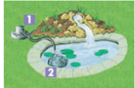
Diagram showing ideal set-up for small pond. 1-Out-of-water filter, 2-Solids handling pump. Out of water filters are easier to clean and maintain. If you use a pump requiring a prefilter, the prefilter ends up doing all the work and frequently clogs, requiring extra maintenance. The correct pump for this situation is one that does not require a prefilter and comes in flow rates appropriate for the capacity of the out-of-water filter.
