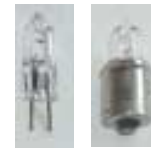
T-type Halogen Bi-pin/Bayonet Shown half size. 10-75 watts 2-3,000 hours (avg) Most often used in reflector floods, step, and spotlights.
