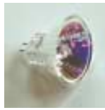
MR-11 Halogen Bi-pin Shown 1/4 size. 10-50 watts 2-3,000 hours (avg)
