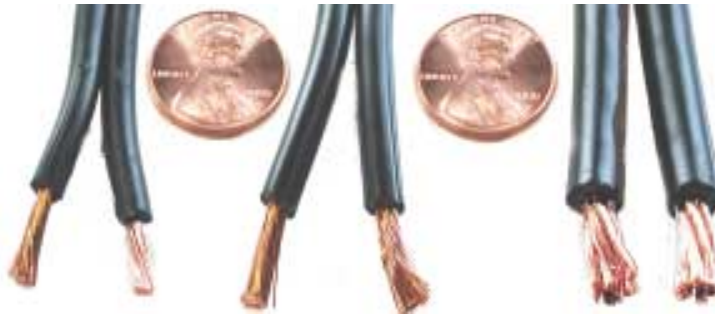
Shown actual size, (l to r) 12 gauge, 10 gauge and 8 gauge. Low voltage lighting cable is UV resistant and suitable for direct burial. It is often easier to use two runs of 12 or 10 gauge than deal with the huge girth of 8 gauge cable.
