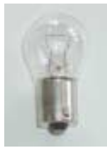
Single/Double Contact Incandescent Shown half size. 6.9-29 watts 700-2,000 hours (ave) Used mainly in pathlights and area lights.
