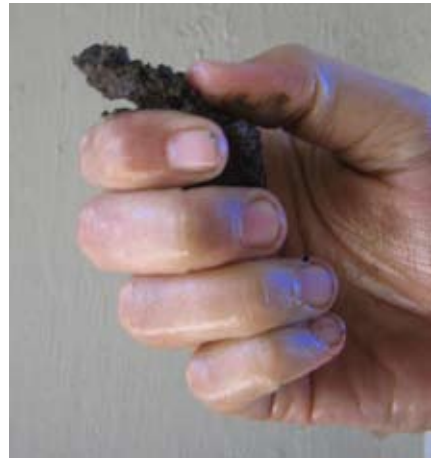
Soil ribbon being squeezed between thumb and finger. Photo: Josh Lowe.
